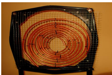
Fig. 2. Copper coil wounded on Front panel of fan
